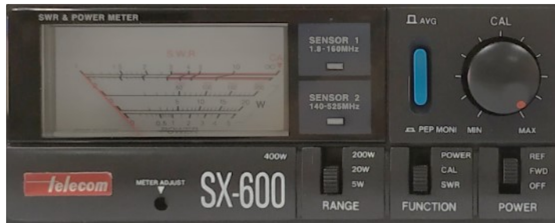
Example of an SWR meter
